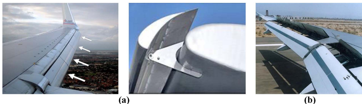
Fig. 1. Similar to an airplane landing and takeoff mechanism, aerodynamic features are inspired to reduce wind uplift loads: (a) slats (leading edge), and (b) flaps (trailing edge).
