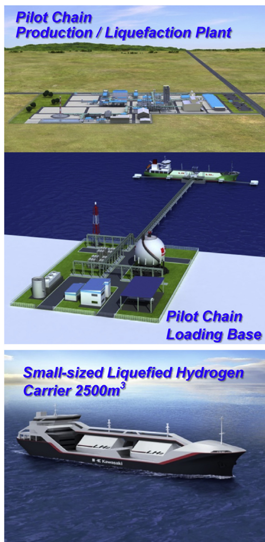
Fig. 1 – Small-scale pilot CO 2 -Free Hydrogen Supply Chain (production plant, loading base and small-sized liquefied hydrogen carrier).
