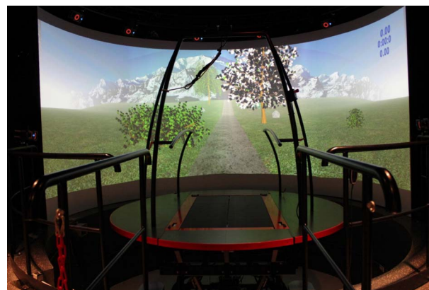
Fig. 1. Virtual environment with a treadmill motion base and 180° cylindrical display.
