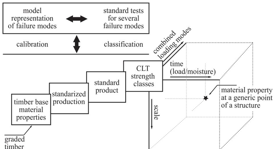
Fig. 1. Strength and stiffness related properties are relevant to represent in structural design assessment. However, this includes the consideration of various aspects.
