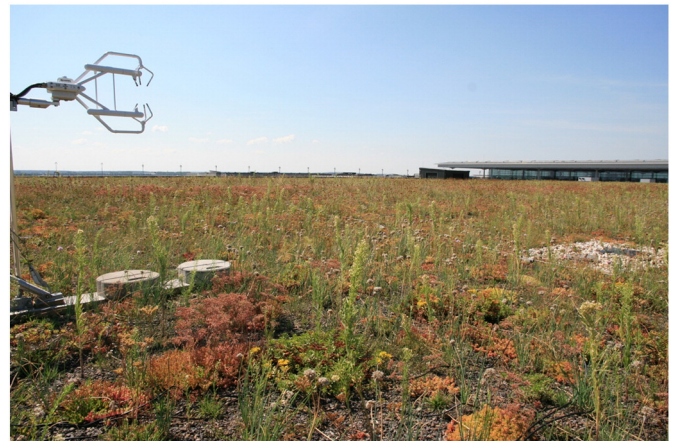
Fig. 1. The BER green roof in the summer period showing parts of the eddy covariance setup (sonic anemometer and open-path gas analyser). The photograph was taken on 22 July 2014. (For interpretation of the references to colour in this figure legend, the reader is referred to the web version of this article.)
