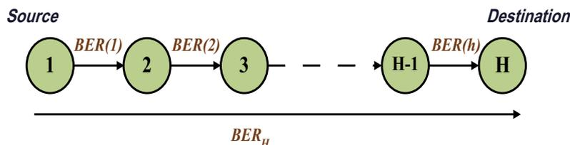
Fig. 1. Multi-Hop Path with H node, Individual BER associated at the hop from node 1 to node H. BER end to end from node 1 to node H.
