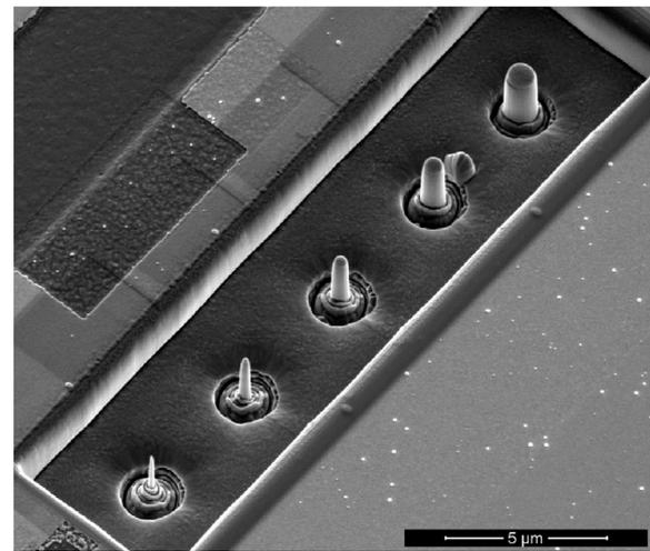
**Fig. 1.** SEM image of an array of nanopillars with diameters of 1000, 700, 500, 300 and 150 nm milled in a Ni–Mn–Ga single crystal (alloy A3). The image was taken under a tilt of  $30^\circ$ .
