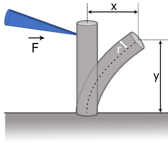
**Fig. 2.** Schematic of the bending deformation of a pillar with the applied force,  $F$ , from the nanomanipulator.
