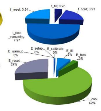
Measured: 1.98 kWh/kg
