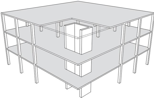
Fig. 1. Core wall in a reinforced concrete structure.
