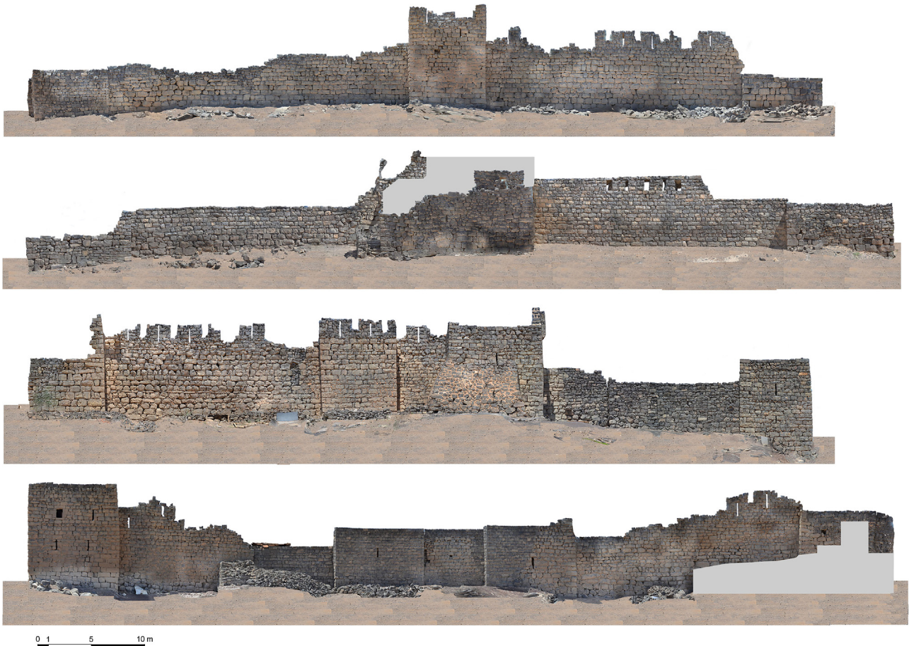
Fig. 2. Photogrammetry of the external walls of Azraq castle: a: northern external elevation; b: western external elevation; c: southern external elevation; d: eastern external elevation. Parts that it was not possible to process in grey. Photogrammetry: Marta Tenconi.
