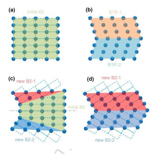
Schematic drawing of the formation of special grain boundaries in B2 during transformation cycling ( $\{011\}$  cross-section of B2 with only one set of sub-lattice atoms plotted): (a) perfect crystal in initial B2 state; (2) compound twinning in B19' states; (3)  $\Sigma$ 9 boundaries between the initial B2 and new B2 states; (4)  $\Sigma$ 3 boundary between two new B2 states.
