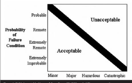
Figure 1. EASA Acceptable Means of Compliance 25.1309: probability versus severity.
