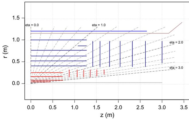
**Fig. 1.** Baseline layout of the new inner detector for the Phase II upgrade [7]. Pixel (strip) layers and discs are indicated in red (blue). (For interpretation of the references to color in this figure caption, the reader is referred to the web version of this article.)
