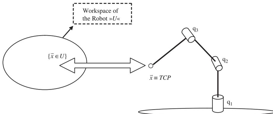
Fig. 1. The position of the robot and a point in the workspace.
