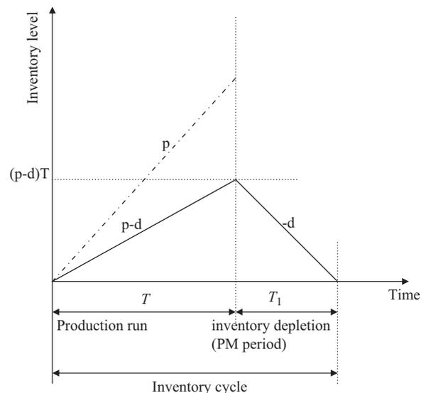
Fig. 1. The inventory cycle of the EPQ model with inventory building and depletion period.
