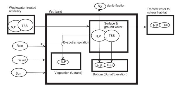
Fig. 1. Diagram of the wetland treatment method. Wetlands remove nutrients and retain suspended solids by physical settling, chemical precipitation, adsorption, and biological metabolism. The processes are controlled by natural energies such as sunlight, wind, and rain. Permanent nutrient pathways are burial, vegetation uptake, and denitrification.
