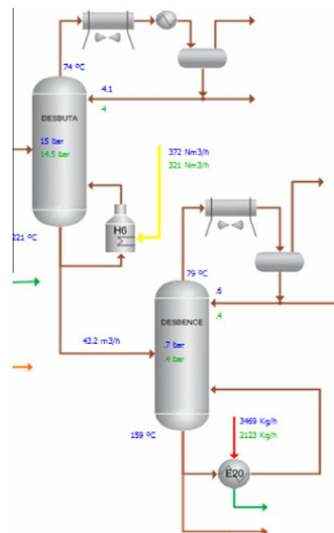
Fig. 1. Flow diagram of the distillation unit.
