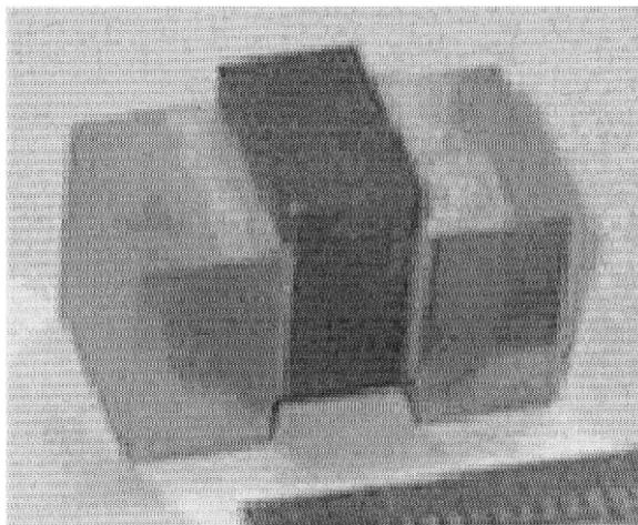
Fig. 1. View of a mechanical test sample W/SiC/W.
