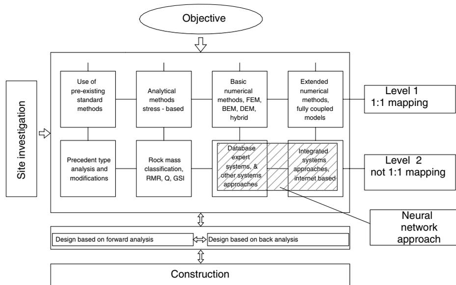
Fig. 1. The four basic methods, presented in two levels which comprise eight different approaches to rock mechanics modeling [2].
