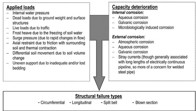
**Fig. 2.** Summary of CI pipe structural failure mechanisms.
