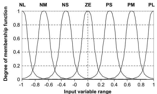
Fig. 1. Membership functions used for input and output variables of the proposed FLC.
