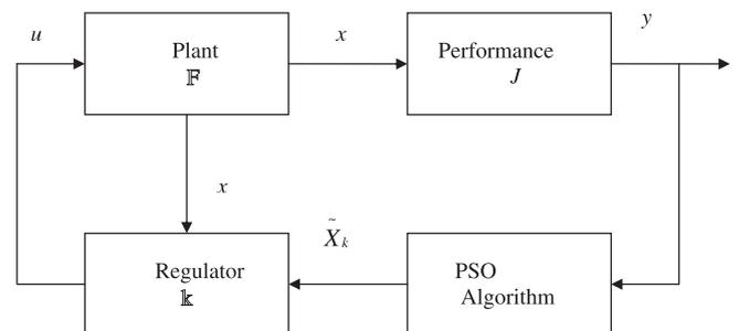
Fig. 1. PSO-based extremum seeking block diagram.
