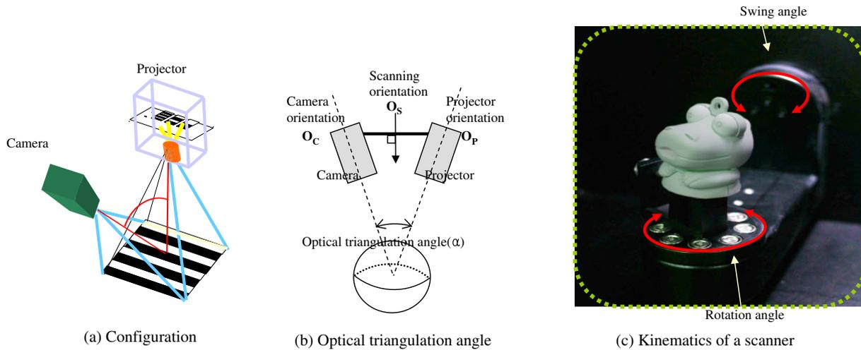
Fig. 1. SLS mechanism.
