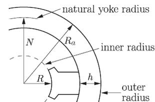
Fig. 1. Simplified analytical model of IM with teeth.
