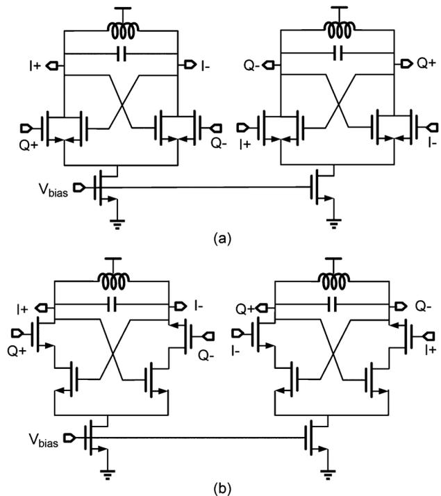
Fig. 1. Schematic of traditional QVCOs. (a) P-QVCO. (b) S-QVCO.
