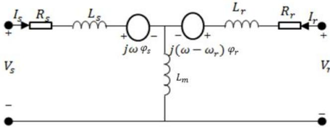
Fig. 2. DFIG electric equivalent model
