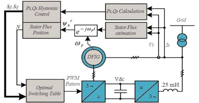
Fig. 3. DPC scheme for DFIG grid connection
