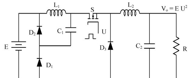
Fig. 1. Quadratic buck converter with a single switch.
