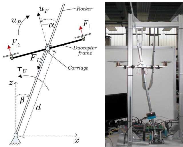
Fig. 1. Mechanical structure and corresponding test rig.
