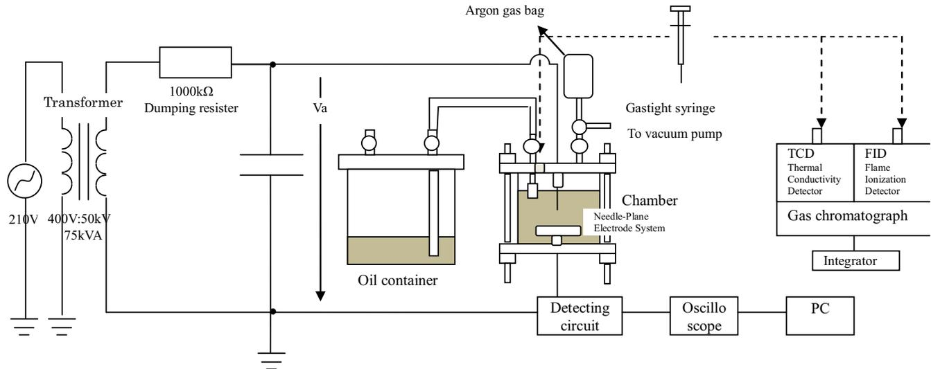
Figure 1. Diagnostic system to generate and measure PD [7].
