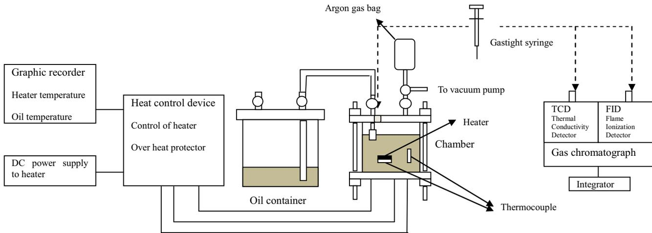
Figure 2. Diagnostic system to generate and measure overheating.
