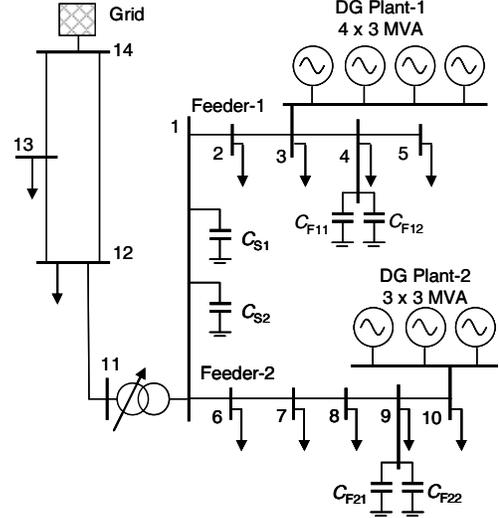
Fig. 2. One-line diagram of the system under study.
