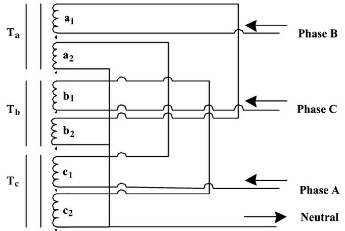
Fig. 2. Zig-zag transformer for neutral current compensation.
