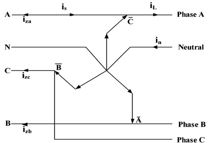
Fig. 3. Diagram showing the flow of currents of zig-zag transformer for neutral current compensation.
