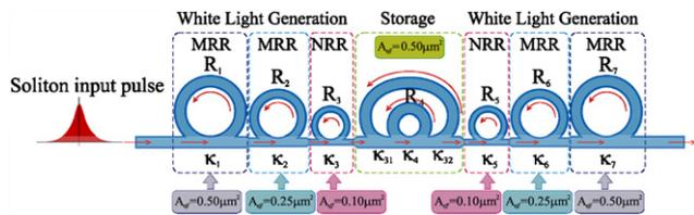
**Fig. 1.** A schematic of an upstream and downstream white light generation system with a storage unit, where  $R_i$ : ring radii,  $\kappa_i$ : coupling coefficients, MRR: micro-ring resonator, NRR: nano-ring resonator.
