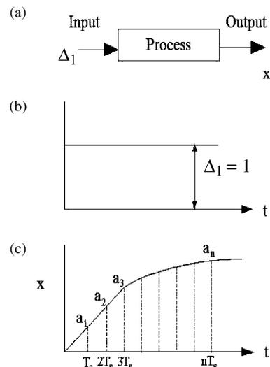
Fig. 3. Dynamic matrix coefficients of a process.
