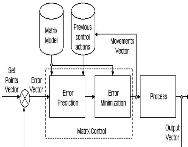
Fig. 1. Architecture of a DMC controller.
