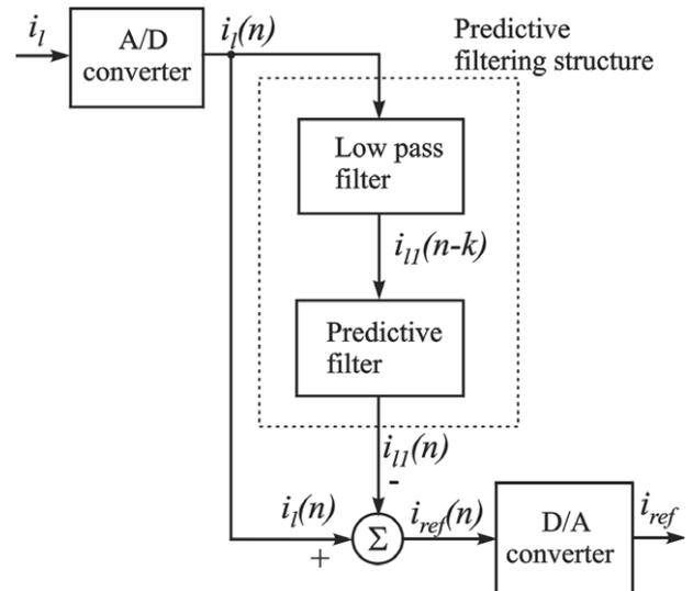
Fig. 2. Block diagram for current reference determination.
