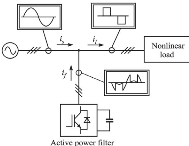
Fig. 1. Block diagram of an active power filter.
