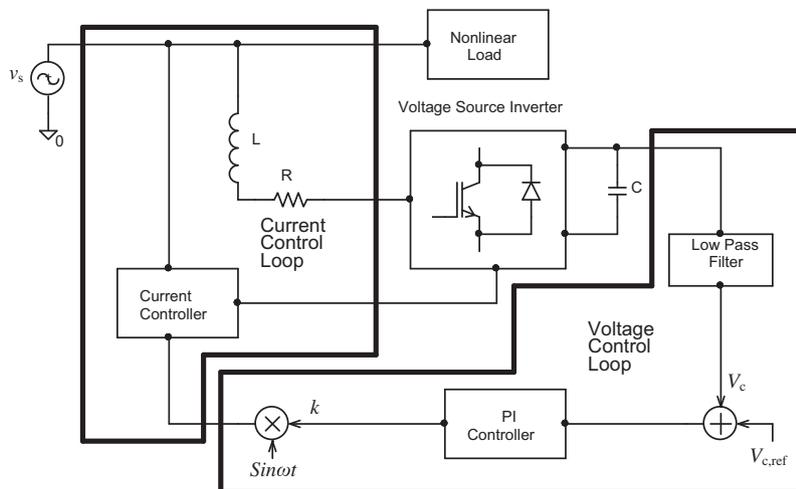
Fig. 1. Indirect current controlled shunt APF.
