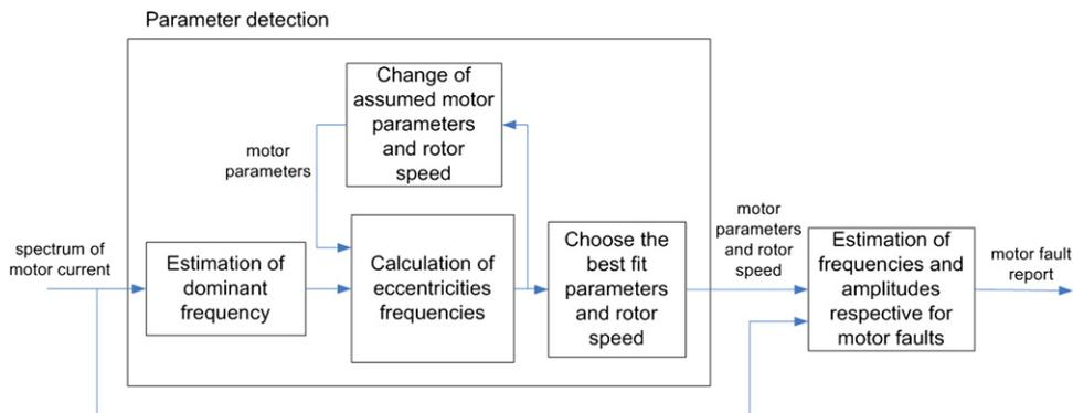
Fig. 1. Motor parameters and rotor speed detection scheme.
