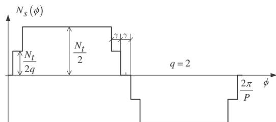
Fig. 2. Winding distribution. Particular case with  $q = 2$ .
