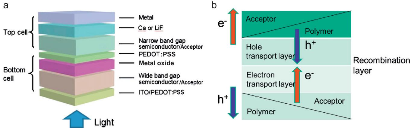
**Fig. 1.** (a) Device configuration of a typical double junction polymer solar cell and (b) the mechanism of the interfacial layers consisting of HTL and ETL. The HTL is typically PEDOT:PSS, while ETL is  $\text{TiO}_2$ ,  $\text{ZnO}$  or  $\text{Nb}_2\text{O}_5$ .
