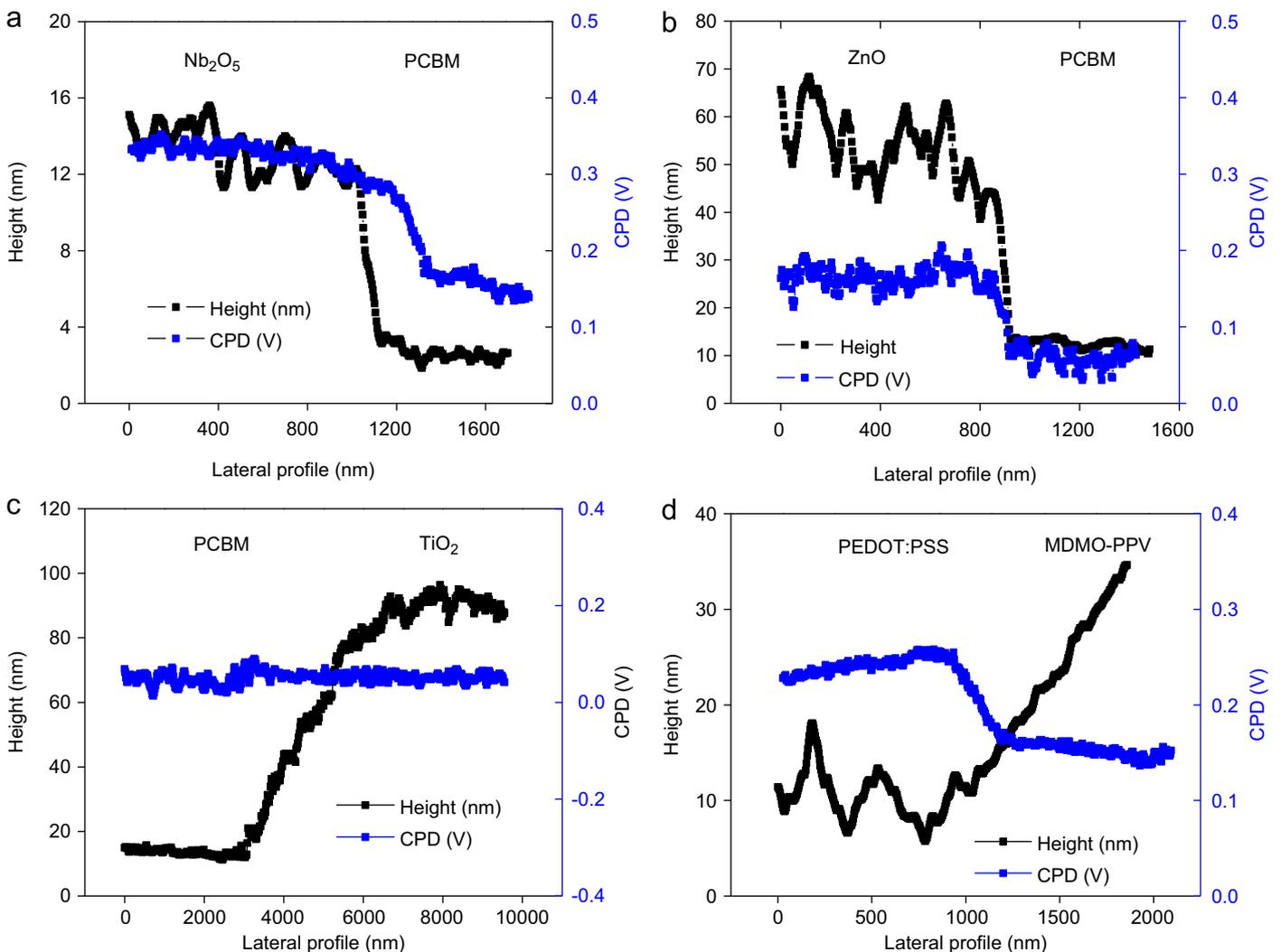
**Fig. 2.** Height and surface potential across a surface interface measured by scanning probe microscope (SPM) of (a)  $\text{Nb}_2\text{O}_5$  on top of PCBM, (b)  $\text{ZnO}$  on top of PCBM, (c)  $\text{TiO}_2$  on top of PCBM, and (d) MDMO-PPV on top of PEDOT:PSS.
