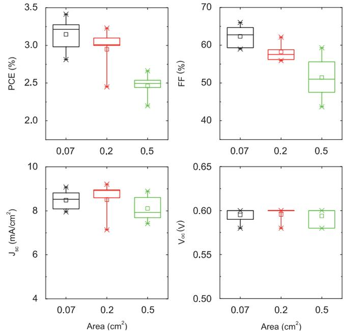
**Fig. 2.** Statistics for PCE, FF, *J*<sub>sc</sub> and *V*<sub>oc</sub> as functions of device area.
