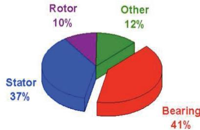
Fig.1. Study of statistics faults in induction motors.
