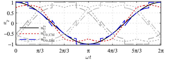
Fig. 2. Modulation functions for continuous (CM) and discontinuous (DM) modulation
