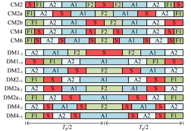
Fig. 3. Pulse pattern of the implemented modulation methods, S = Shoot-Through state, A1, A2 = Active states, F1, F2 = Freewheeling states
