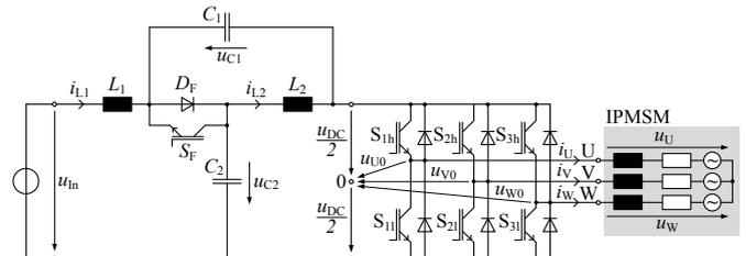
Fig. 1. Lossless QZSI with IPMSM
