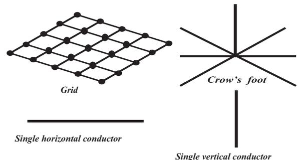
Fig. 1. Representation of a grounding system by single conductor, or by interconnected conductors.
