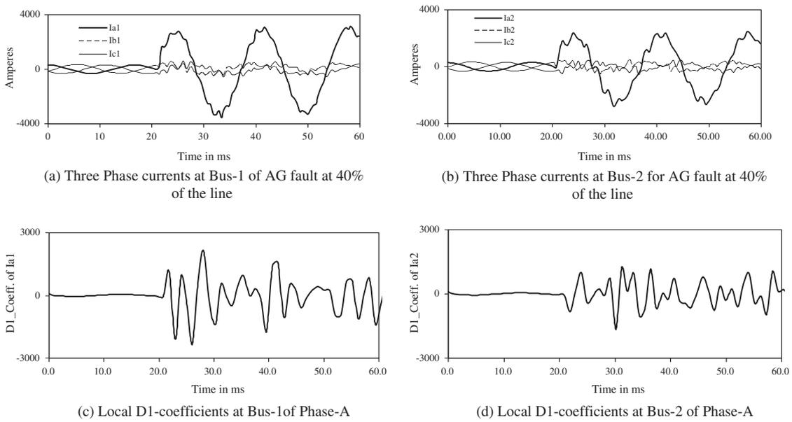
Fig. 2. Fault current transient and their detail coefficients.
