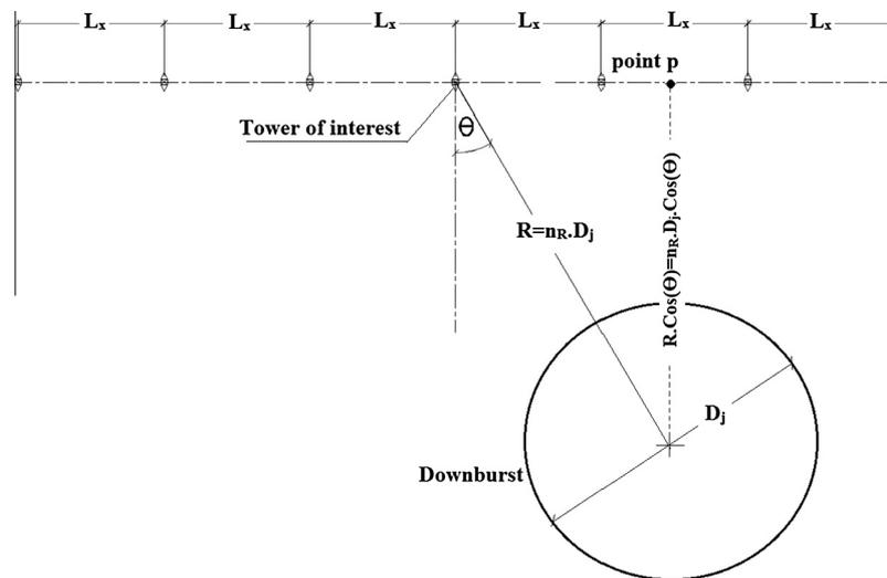
Fig. 1. Downburst parameters.
