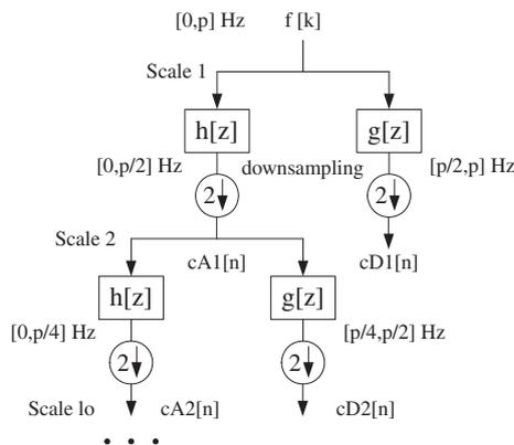
Fig. 1. Wavelet filters bank.
