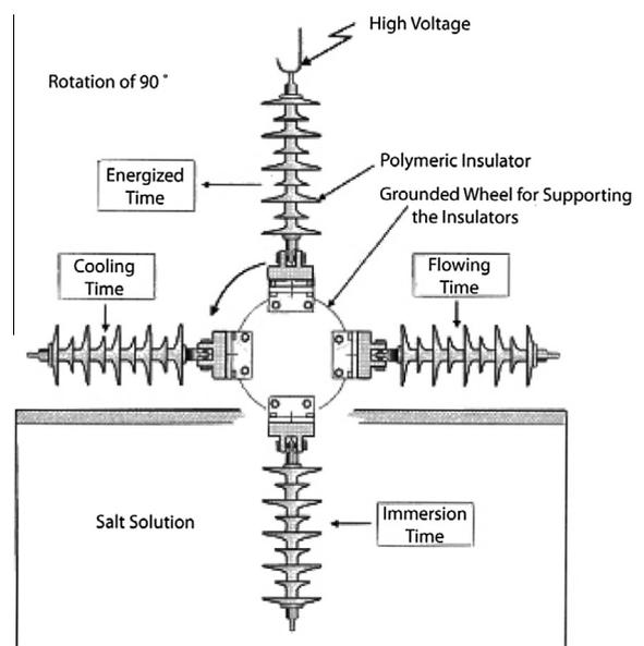
Fig. 1. Schematic illustration of the electric tracking wheel.
