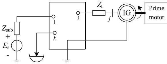
Fig. 1. Equivalent circuit of IG in grid.
