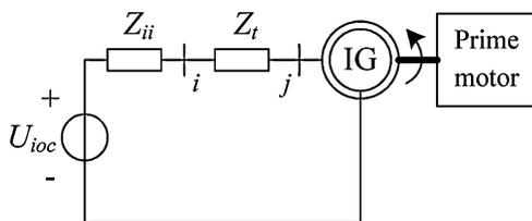
Fig. 2. Thevenin equivalent circuit of node  $i$ .
