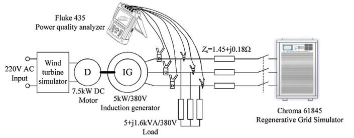
Fig. 3. Laboratory setup for voltage flicker measurement.
