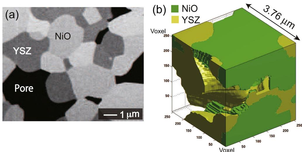
**Fig. 1.** (a) 2D FIB-SEM image and (b) corresponding 3D reconstruction of composite NiO-YSZ anode before reduction. (Green: NiO Gray, yellow: YSZ). (For interpretation of the references to colour in this figure legend, the reader is referred to the web version of this article.)
