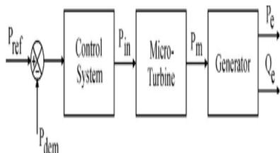
Fig. 1 Micro-turbine model
