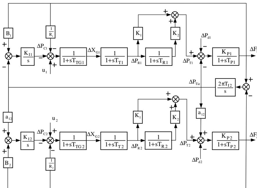
Fig. 1. Block diagram of a two-area power system.
